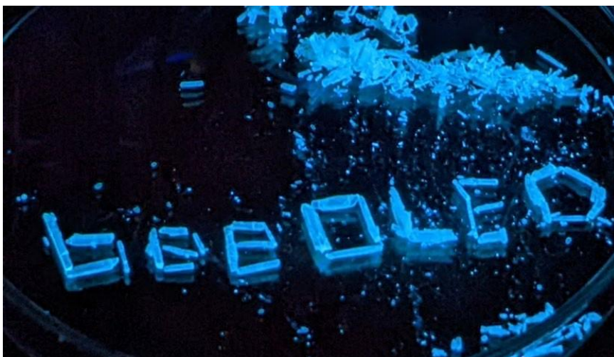
Perfect crystals grown for XRD (X-ray structure analysis). Deep blue light is emitted under UV light irradiation.
